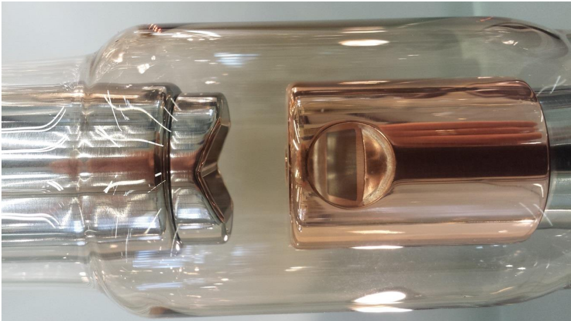
Figure 24 Close-up photo of the Philips superimposed dual focal spot stationary anode tube FO 17 for surgical C-arm systems.
