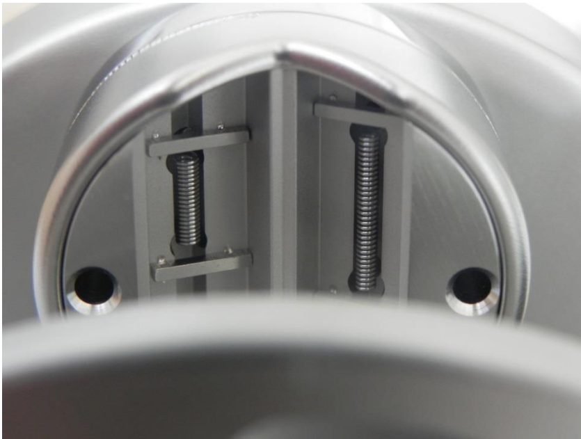
Figure 32 Close-up view of the thermionic cathode for superimposed focal spots of a Philips SRO™ 33 100 tube.
