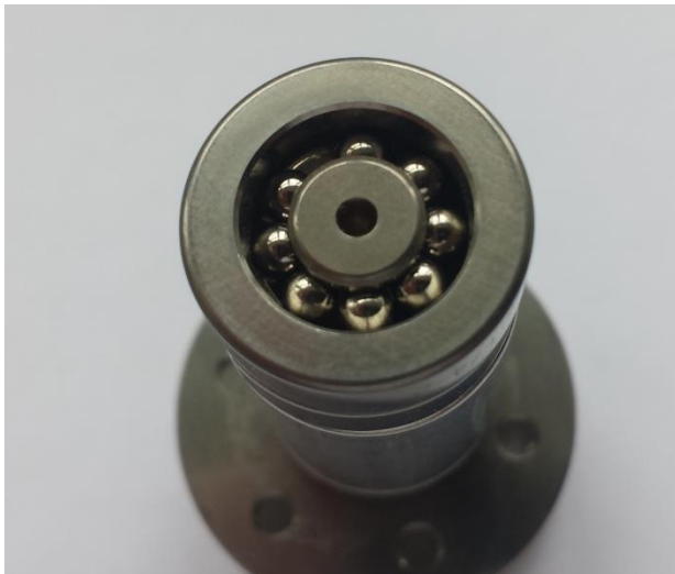
Figure 33 Ball bearing system for Philips SRO™ tube series tube with 90 mm target diameter.
