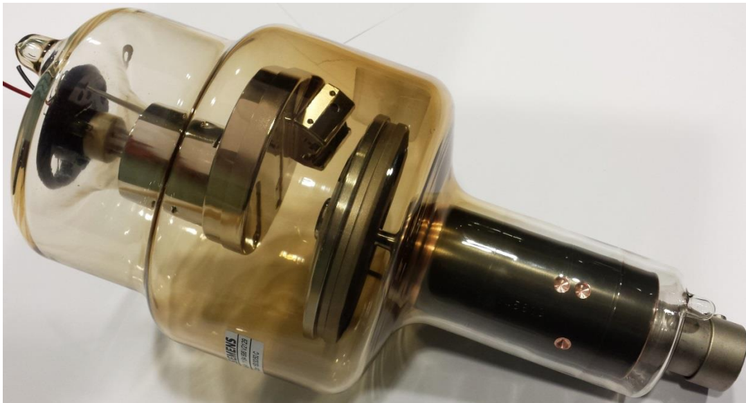
Figure 20 Brazed graphite-backed RW/TZM compound anode in a Siemens Opti 150 30 50 radiographic tube.
