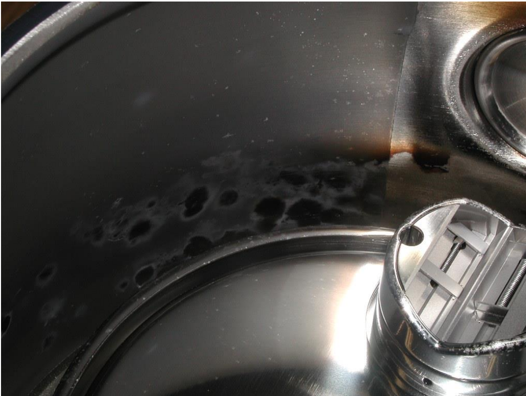
Figure 45 Traces of arcing between metal electrodes of a metal center section tube for angiography. A glass wall would have imploded under such severe arcing.
