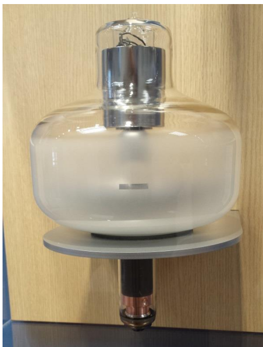
Figure 40 Frosted glass wall of a tube from Dunlee, Aurora, IL, USA, subsidiary of Philips, to improve the electrical stability under bombardment by backscattered electrons.
