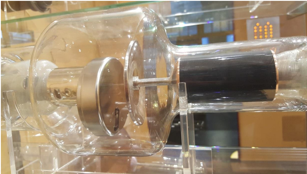
Figure 31 Hidden cathode in a Philips tube from the production plant in Eindhoven, The Netherlands. (Picture taken at the Medizinhistorisches Museum Hamburg, Germany, UK.)
