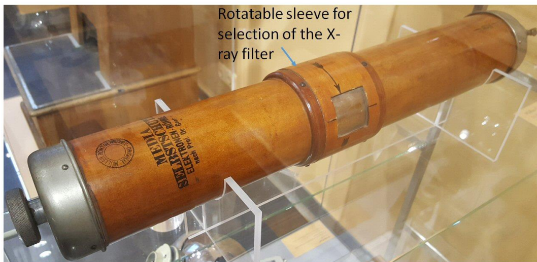
Figure 14 “Fully protected” Philips Media™ tube from the 1920ies. A rotatable sleeve allowed for selecting the X-ray filter thickness. (Photo taken at the Medizinhistorisches Museum Hamburg, Germany, UKE.)
