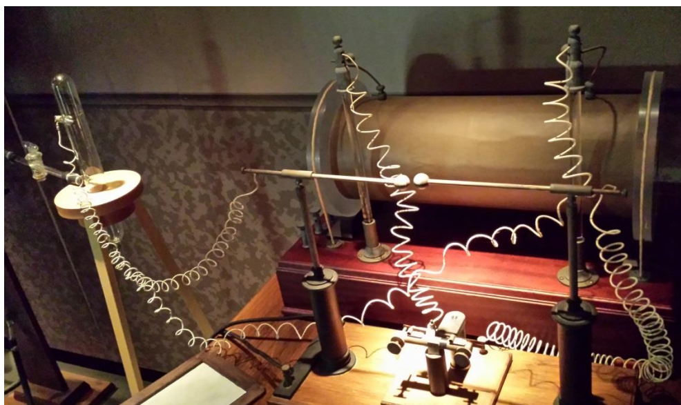
Figure 1 Replica of C.W. Röntgen’s first experimental equipment in his laboratory in Würzburg, Germany. It shows an actively pumped simple Crookes tube and a “large” Ruhmkorff inductor. Röntgen discovered X-rays at dawn of Friday November 8 th , 1895. (Photo taken at the German Röntgen Museum, Remscheid-Lennep, Germany.)
