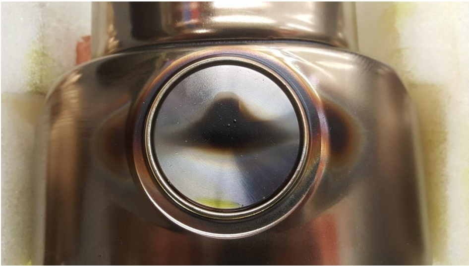
Figure 44 Carbonized beryllium X-ray window after impact of electrons backscattered from the focal spot of a bi-polar angiography tube.
