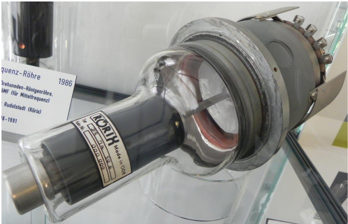
Figure 48 Mammography tube with metal center section, cathode grounded, produced between 1980 and 1991 by VEB Rudolstadt (Rörix, later Siemens), Rudolstadt, GDR.(Photo taken in the Siemens X-ray tube museum Rudolstadt, Germany.)
