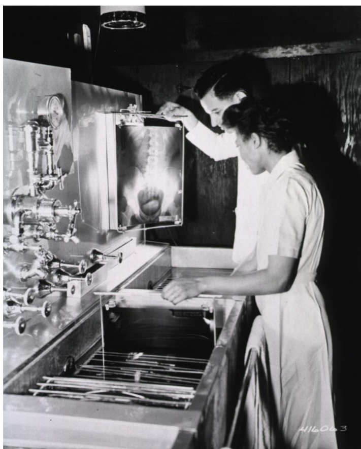
Figure 4.a Radiographs recorded on a glass plates being chemically processed. They are rigid, fragile, and relatively heavy to handle b. An early radiograph recorded on a glass plate.
